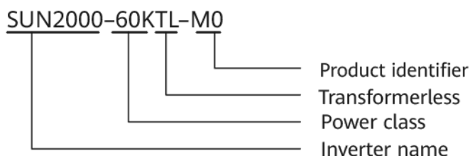
Figure 2-1 Designation explanation of the SUN2000-60KTL-M0
